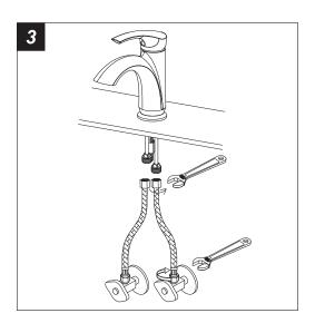
3. Connect the flexible hoses to the water supply valve and copper tubes. Tighten it with the adjustable wrench.
